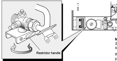
Rotate the restrictor handle anti-clockwise to increase temperature and clockwise to decrease temperature as indicated on the handle.
