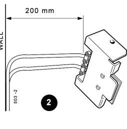
Note. Ensure that the lengths of the current conductors are shorter than the earth conductor so that if the cable slips in its anchorage the current carrying conductors become taut before the earth conductor.
