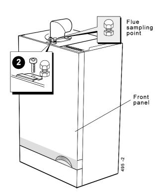
3. Remove the screws and pull out the tabs from the slots.
