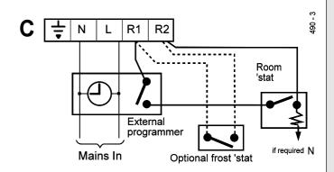
**N.B.** These diagrams are schematic only and do not show external terminal strips etc.
