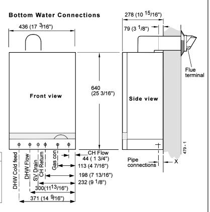
Distance X is 20mm for DHW pipes & safety valve outlet. Distance X is 23.5mm for CH pipes & gas inlet.
