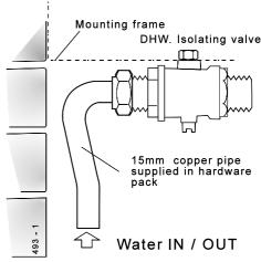
For top connections: use 15mm straight pipe and elbow (not supplied).
