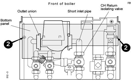
View of underside of boiler
