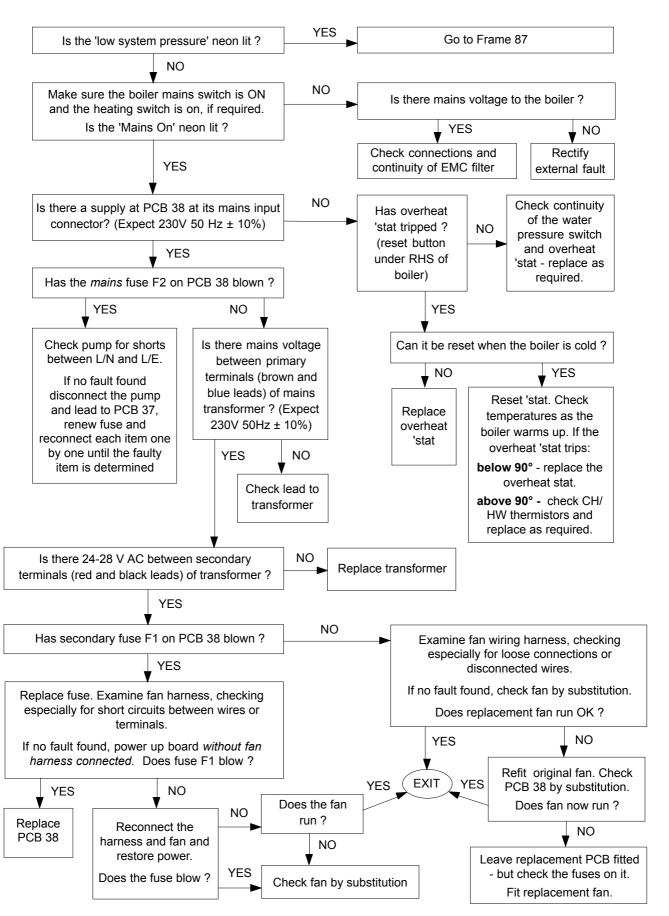
**Foot Note:** Presence of live supply on a terminal may be checked with a multimeter set to the appropriate AC range (apply the other probe of the meter to mains neutral, e.g. on terminal N of the programmer terminal strip).
