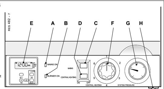
Check that the overheat thermostat has not tripped - press button (H) to reset.
