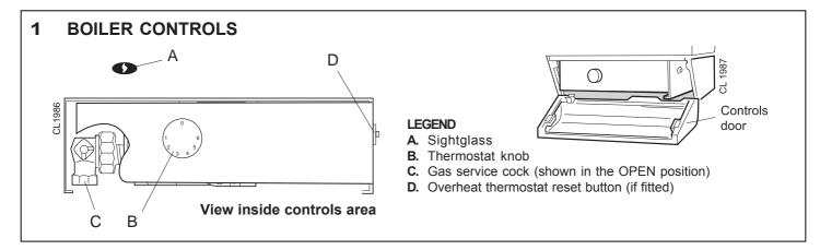
Winter conditions, i.e. central heating and domestic hot water, the thermostat should be set at position 5 or 6.
