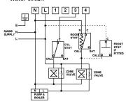
6. Fully Pumped System using RoomStat and Two (2 Port) Spring Return Zone Valve with Auxiliary Switches
