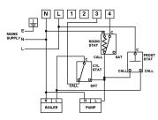
3. Gravity Hot water with Pumped Heating via RoomStat and CylinderStat including Frost protection via double pole FrostStat
