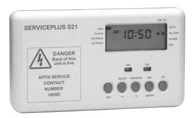
The Horstmann ServicePlus S21/S21R is a 24 hour programmer allowing independent timing of hot water and central heating with up to 3 ON/OFF settings per 24 hours and a hot water boost button and central heating advance override.
