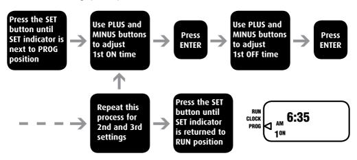
NB. The factory default settings for the 2nd ON/OFF times are both set at 12:00pm (midday) which cancels this 'ON' period giving 2 ON/OFF periods for 24hrs. If a midday 'ON' period is required set the 2nd ON and OFF times accordingly. If not press ENTER twice.
