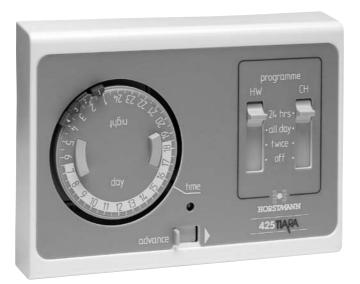
The Horstmann 425 Tiara and Diadem programmers are 2 circuit central heating and hot water programmers able to switch ON and OFF twice every 24 hours. An advance switch is provided to make temporary overrides to the ON or OFF periods and a selector switch gives a further choice of programmes.
