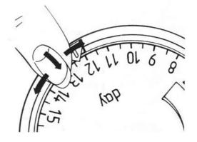
Please ensure the clock is set to the correct current time after altering the ON/OFF settings.
