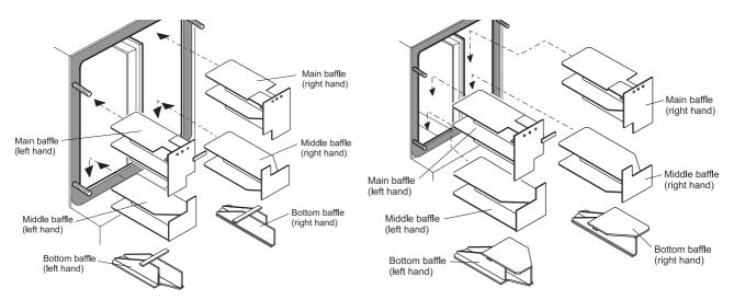
Fig. 24 - Combi 90 V3 baffle positions
