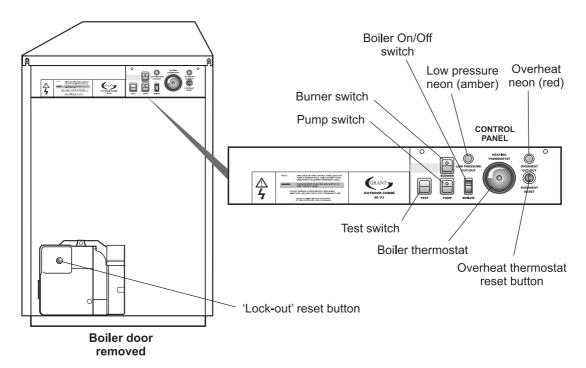
Fig. 21 - Boiler controls (Outdoor Combi 90 V3 and Combi MAX)
