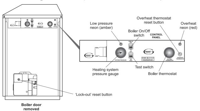
Fig. 22 - Boiler controls (Outdoor Vortex Combi)
