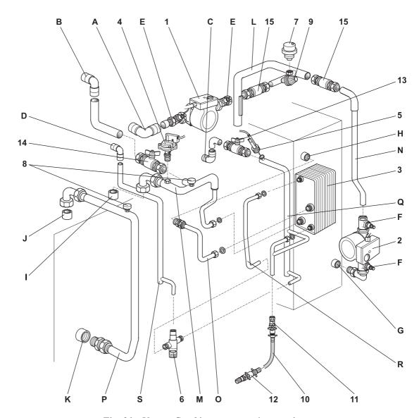
Fig. 31 - Vortex Combi components/connections
