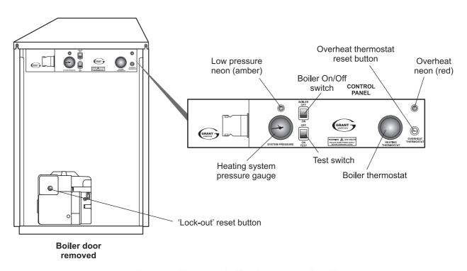
Fig. B - Boiler controls (Outdoor Vortex Combi)
