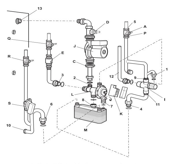
Fig. 30 - Combi 90 V3 and Combi Max components/connections
