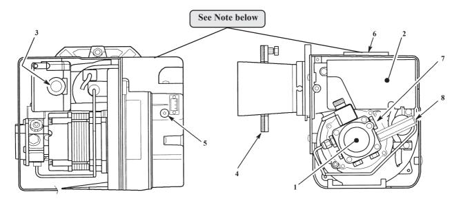
Fig. 20 - RDB burner components
