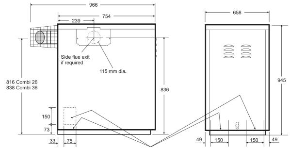
2 holes 75 x 150 mm in base and each side of boiler enclosure covered with movable plates
