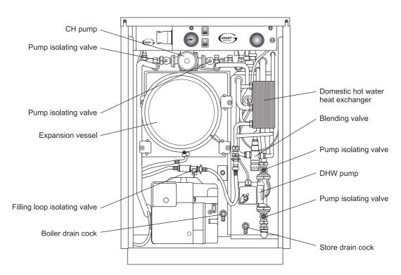
Fig. 23 - Outdoor Vortex Combi components
