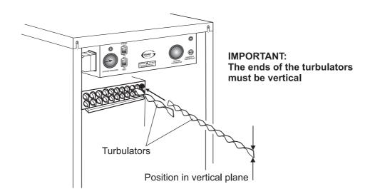
Fig. 28 Outdoor Vortex Combi turbulators
