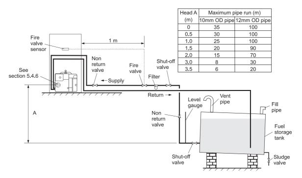
Fig. 6 - Two pipe system
