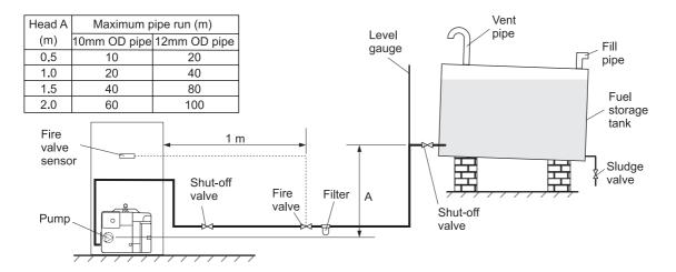
Fig. 5 - Single pipe system
