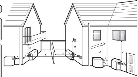
Fig. 11 - Flue terminal positions
