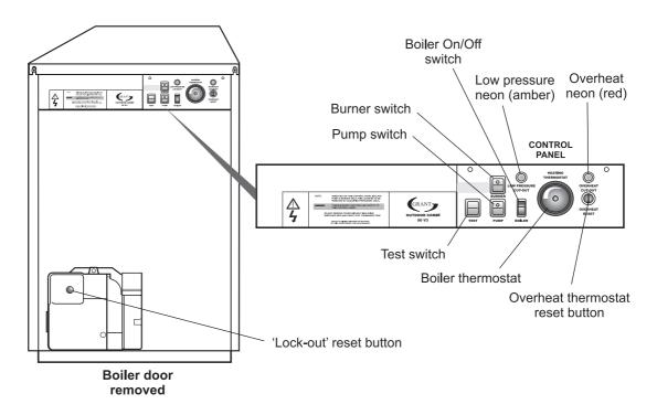
Fig. A - Boiler controls (Outdoor Combi 90 V3 and Combi MAX)
