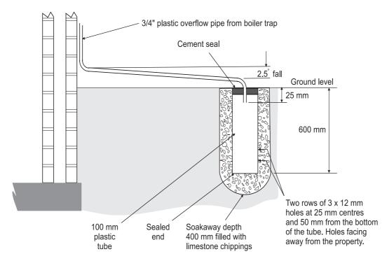
Fig. 14 - Purpose made condensate soakaway
