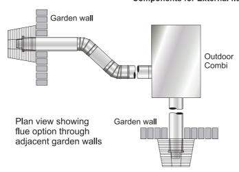
Fig. 16 - Outdoor high level flue (Green system)
