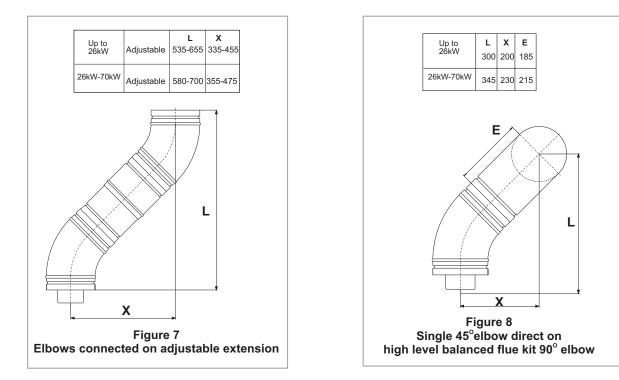
High Level Balanced Flue Kit
