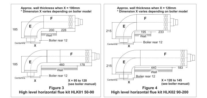
High Level Balanced Flue Kit
