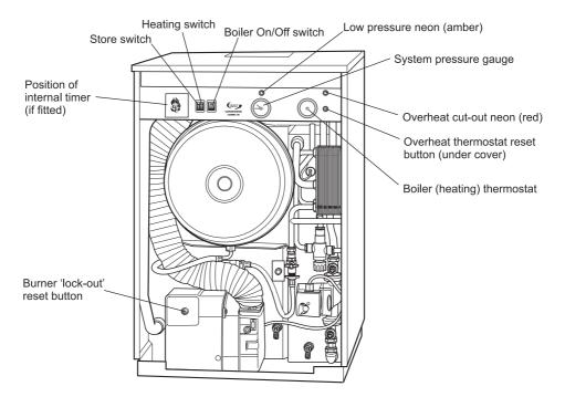
Fig. 25a Boiler controls (Vortex Combi 36 shown)
