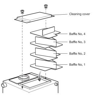
Fig. 26 - Combi 70 V3 baffle positions
