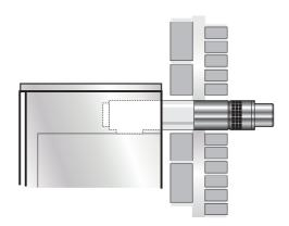
Fig. 20 - Low level balanced flue
