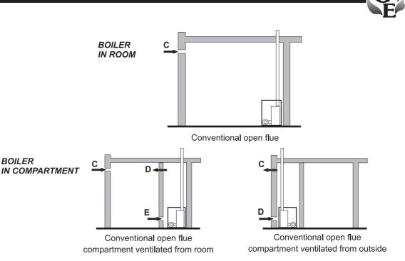
Fig. 11 - Combustion and ventilation air supply for conventional flue boilers
