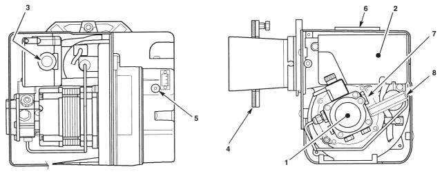
Fig. 24 - RDB burner components
