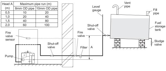
Fig. 5 - Single pipe system
