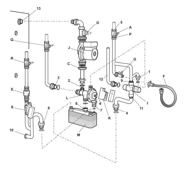
Fig. 33 - Combi V3 and Combi Max components/connections
