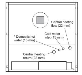
Fig. 22 - Combi V3 and Combi Max pipe positions
