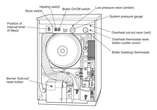
Fig. B - Boiler controls (Vortex Combi 36 shown)
