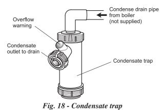
The trap must be located internally in an accessible position to allow for routine maintenance. The mounting bracket supplied with the trap **MUST** be used - the trap should **NOT** be supported by the condensate pipework only.
