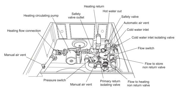
Fig. 22a Vortex Combi pipe positions
