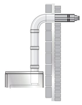
Fig. 21 - High level balanced flue
