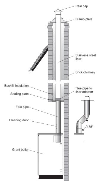
Fig. 12 - Typical conventional flue with brick chimney
