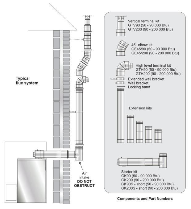
Fig. 14 - External flue (Green system)
