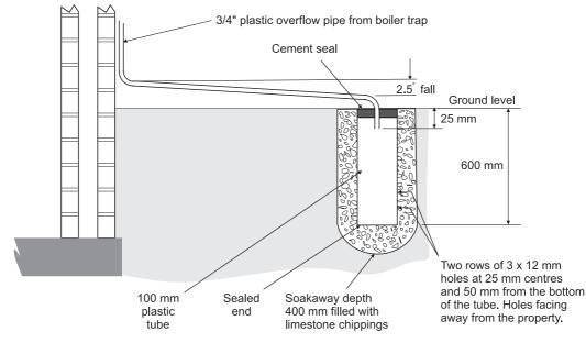
Fig. 19 - Purpose made condensate soakaway
