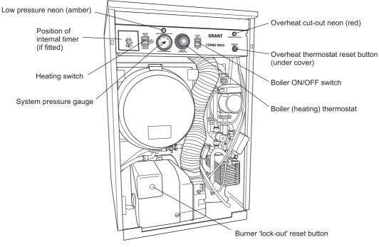
Fig. 25 - Combi V3 and Combi Max boiler Controls
