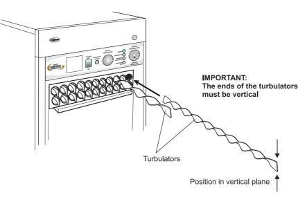
Fig. 31 Vortex Combi turbulators
