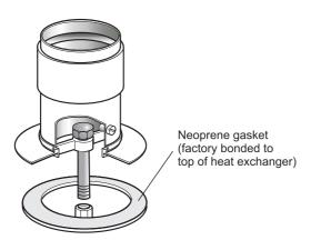
Fig. 23 - Vortex Combi conventional flue adaptor
