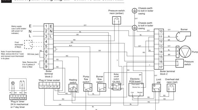
12.1 Control panel wiring diagram - Combi V3 and Combi Max
