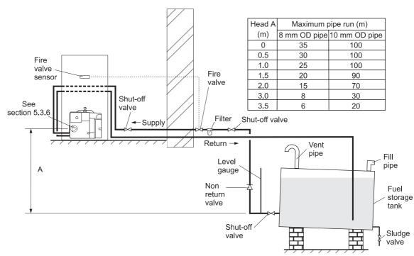
Fig. 6 - Two pipe system
