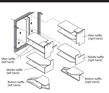
Fig. 28 - Combi Max baffle positions
