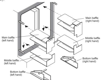
Fig. 27 - Combi 90 V3 baffle positions
