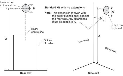
Fig. 21a - High level balanced flue (White system)
