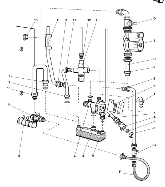
Fig. 38 - Combi 70 water components/connections
