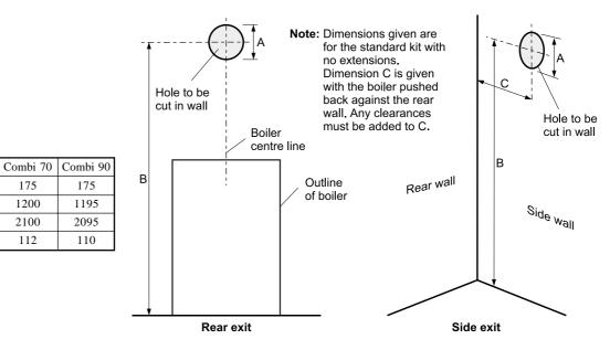
Fig. 14 - High level balanced flue
