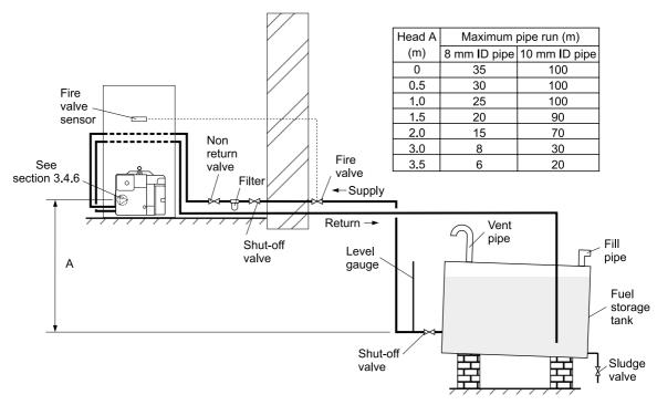
Fig. 4 - Two pipe system
