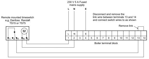
**Important:** If a remote timer is used, it must be a single channel 240V unit incorporating voltage free output contacts.
