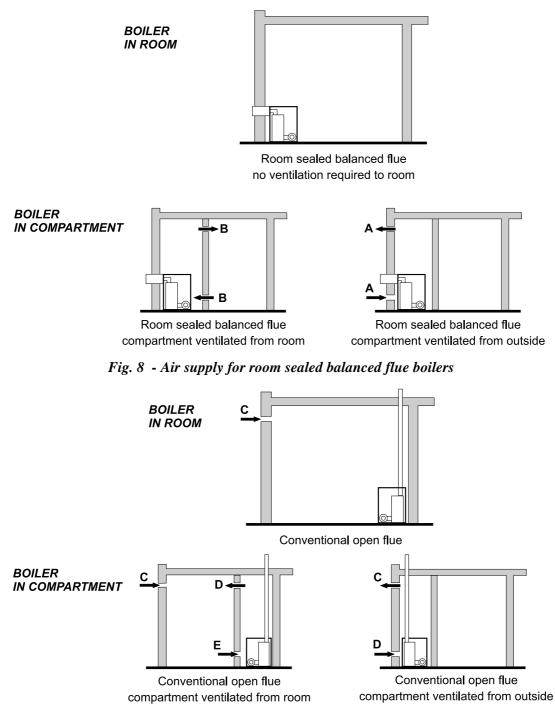
Fig. 9 - Combustion and ventilation air supply for conventional flue boilers
