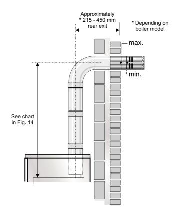
Fig. 15 - High level balanced flue
