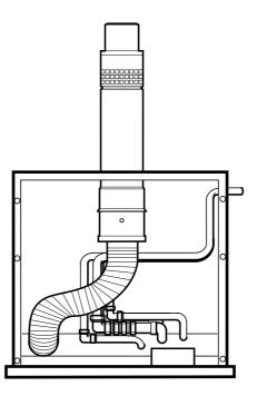
Rear low level flue - Right hand water connections
