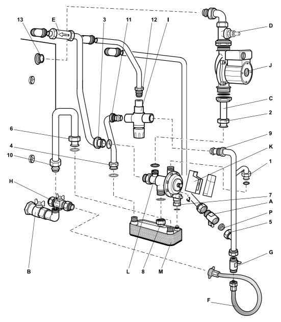
Fig. 39 - Combi 90 water components/connections
