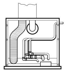
Rear low level flue - Right hand water connections
