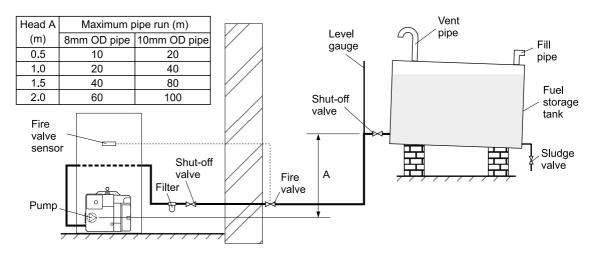
Fig. 3 - Single pipe system
