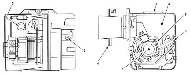
Fig. 31 - RDB burner components
