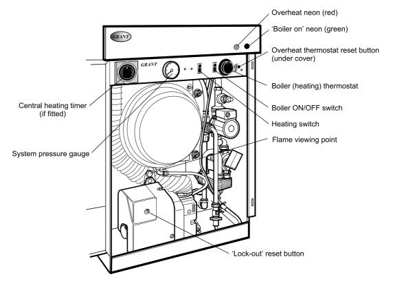
Fig. 32 - shown with pipework cover removed
