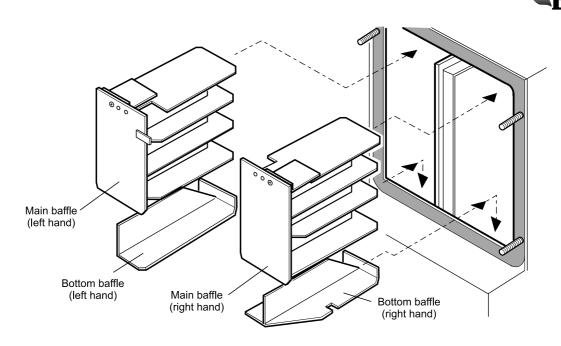
Fig. 34 - Combi 90 baffle positions
