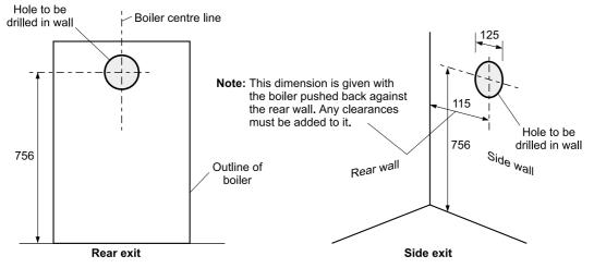
Fig. 13a - Concentric low level balanced flue
