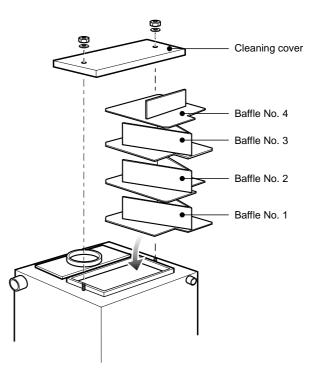
Fig. 33 - Combi 70 baffle positions
