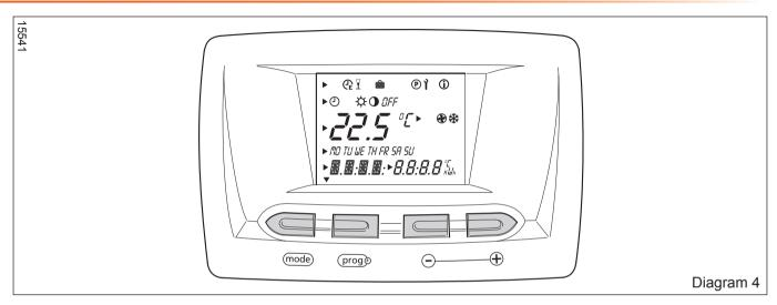
From the basic display you can select and change the major functions by pressing the "mode" button and then the - or + buttons to change their values. By pressing the "mode" button you can move from one menu item to another.
