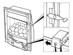
d) Unscrew the burner assembly fixing screws at either side of the firebox, and the two fixing screws at the base of the fire (See fig. 7 below).
