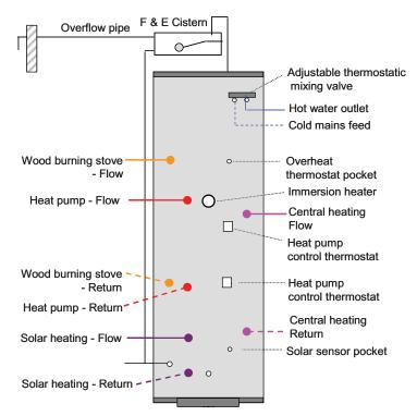
Figure 2 : Torrent MultiFuelStore HP Solar
