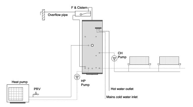
Figure 7: Typical Torrent<sup>HP</sup> system configuration with central heating supplied from a thermal store
