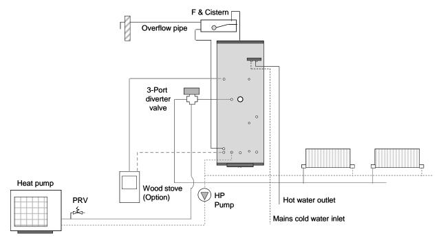
Figure 6: Typical Torrent<sup>HP</sup> system configuration with an optional wood burning stove and central heating supplied directly from the heat pump.
