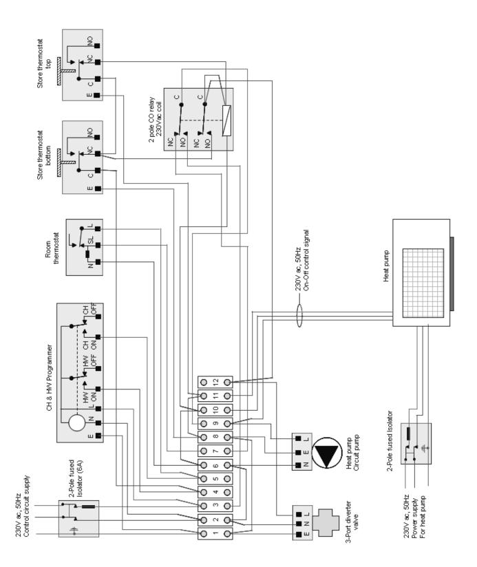
Figure 11 : Typical schematic wiring diagram for the Torrent MultiFuelStore HP and Torrent MultiFuelStore HP-solar with space heating supplied directly from the heat pump circuit as shown in figures 6 & 8.
