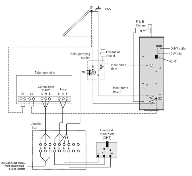
Figure 12 : Typical schematic wiring diagram and system configuration for the Torrent MultiFuelStore HP-solar.
