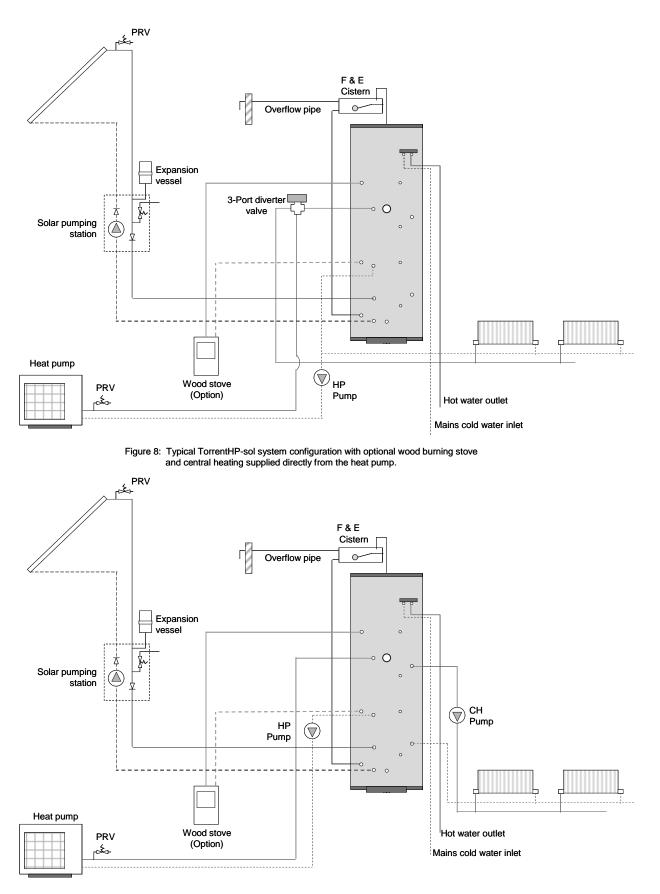
Figure 9: Typical TorrentHP-sol system configuration with wood burning stove option and central heating supplied from the thermal store
