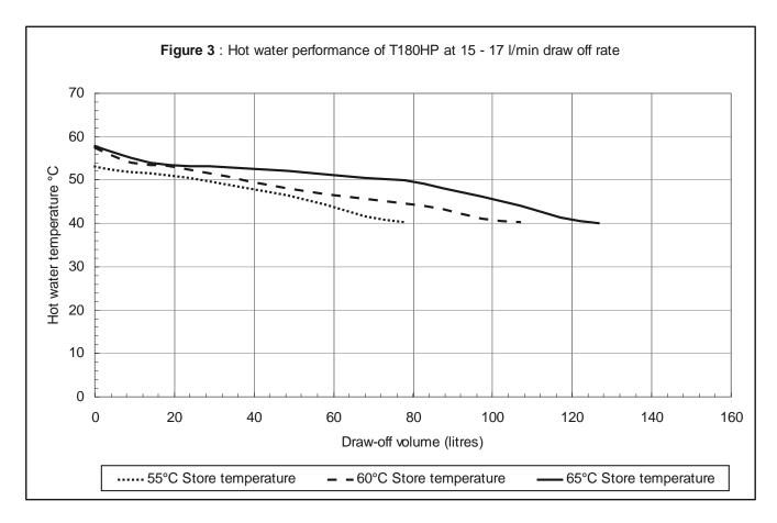
The performance figures shown above for the 180 litre store are increased accordingly as the cylinder capacity increases. The graph illustrates the increase in volumme that can be achieved by the use of the auxiliary heat source.
