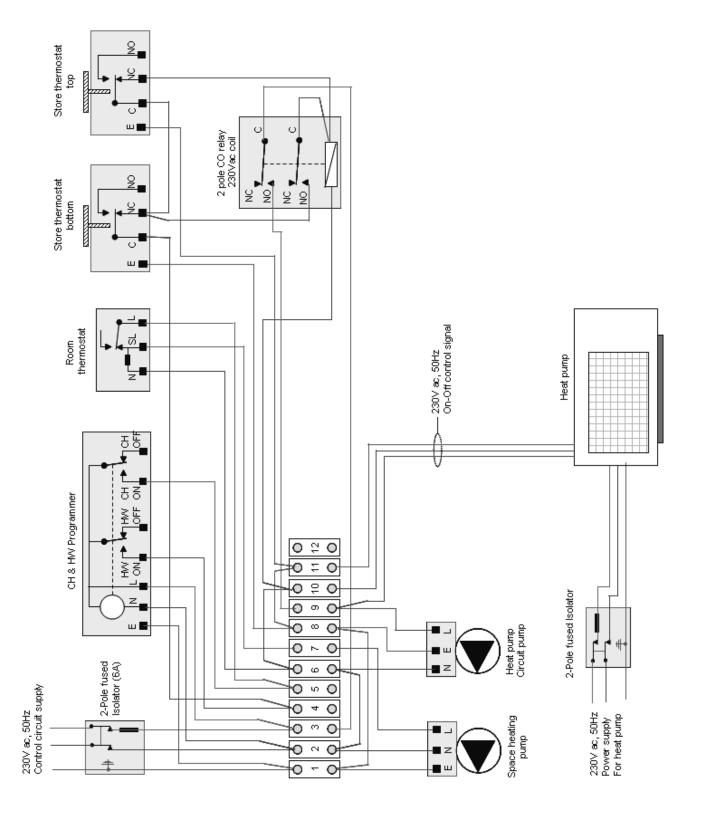
Figure 10 : Typical schematic wiring diagram for the Torrent MultiFuelStore HP and Torrent MultiFuelStore HP-solar with space heating supplied from thermal store as shown in figures 7 & 9.
