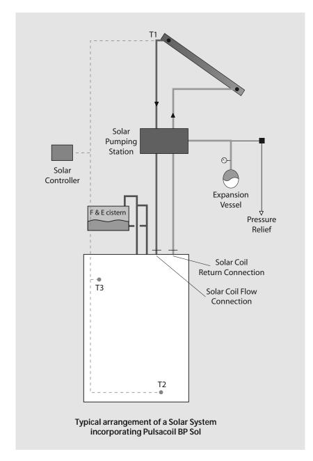
The arrangement and components of a PulsaCoil BP Sol appliance are shown schematically above and on page 4.
