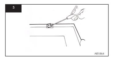
• Lift the glass clear from the lock bracket at the top of the frame and slide out
