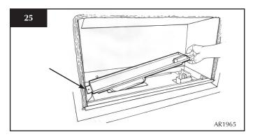
7.5 • Loosen the two screws retaining the plate beneath the burner
