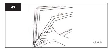
12.2 • Manoeuvre the frame up towards the left side to locate the left hinge pin
