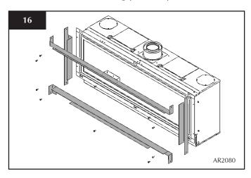
This now determines the width of your two vertical studwork supports. The kit has been designed so that noncombustible board can be taken right up to the edge of the four brackets, Diagrams 17 & 18.
