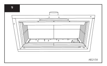
Note: THE HORIZONTAL CHAMFERS MUST ALIGN ON THE REAR AND SIDE PIECES.
