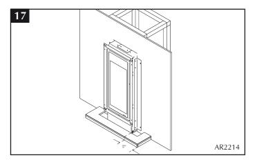
5.5 Attach the retaining brackets to either side of the base section, Diagram 18
