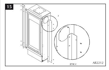
5.3 Attach the retaining brackets to the wall. Use the rawl plugs provided for masonry work, Diagram 16
