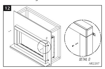
4.9 Cover up the brackets by making good the finish around the fireplace, Diagram 13
