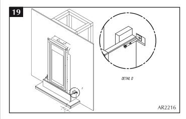
5.7 Attach the side slips by slotting into the cut outs on the base, Diagram 20
