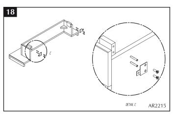
5.6 Secure the base section to the fireplace surround using the brackets, Diagram 19
