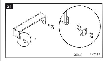
5.9 Locate the top section on the slips, secure the top section to the fireplace surround using the brackets, Diagram 22
