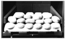
Place the middle row of four pebbles onto the supports in the matrix, over the top of the holes. Ensure the pebbles are not turned sideways, such that they actually enter the holes.
