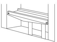
the fire temporarily to check the angle of the baffle. The fret should fit well and the control devices beneath should not be visible to the eye. Realign the baffle if necessary to achieve the correct fit.
