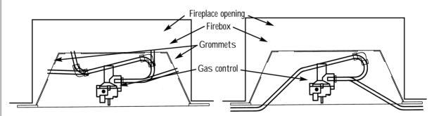
If using an across the hearth connection then the firefront is notched and the supply pipe can be routed through this. The open end of the gas supply pipe should be temporarily sealed to prevent ingress dust and dirt during installation.
