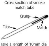
pipe and seal one end. Crimp the pipe to prevent match from sliding down.
