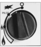
When the pilot lights after the spark keep the knob depressed for approximately ten seconds. Now release the knob and the pilot should stay alight. If the pilot is extinguished during use, wait three minutes before repeating the ignition procedure.
