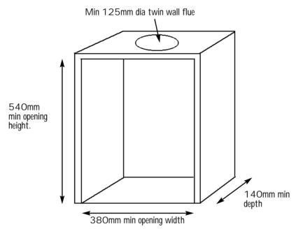
The fire box base and hearth must have a non combustible surface of at least 12 mm thick. The top surface of which must be 50 mm above the surrounding floor or be surrounded by a raised edge or fender 50 mm high.
