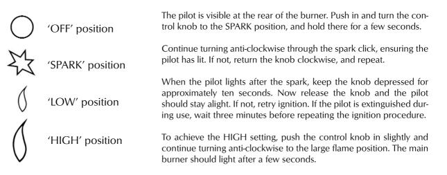
To decrease the setting to LOW, turn the control knob clockwise to the low flame setting. The flame height may be adjusted as desired between high and low settings by turning the control knob to the required position between 'HIGH' and 'LOW'.
