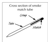
Take a length of 10mm dia pipe and seal one end. Crimp the pipe to prevent the match from sliding down inside
