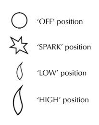
Continue turning anti-clockwise through the spark click, ensuring the pilot has lit. If not, return the knob clockwise, and repeat.
