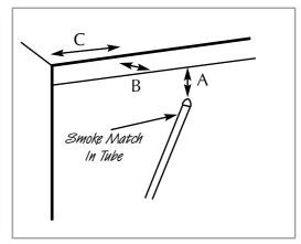
NOTE: If spillage is still indicated after undertaking all of the above, there may be a fault in the flue, or insufficient ventilation is present.
