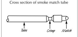
Make a smoke match tube from 10mm diameter tube. Seal off one end and crimp the tube to prevent the smoke match from sliding down inside.
