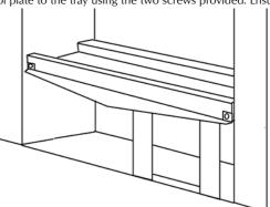
If using an across hearth connection ensure the decorative frame and firefront will clear the supply route. If the data/control plate is not already fitted, attach with two screws, ensuring the control knob is free to be depressed fully.
