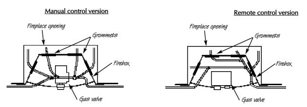
If using a concealed supply it should be laid in accordance with the diagram below. Select the supply route most relevant to the entry point of the gas supply into the fireplace opening. If using an across the hearth connection, then the firefront is notched and the supply pipe can be routed through this.
