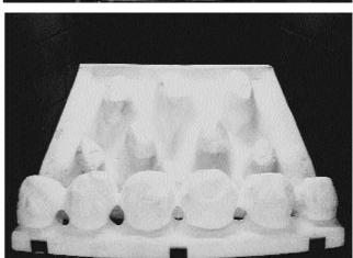
2. Open the bag of 16 ceramic pebbles. All of these pebbles are the same. Take five pebbles and place them as shown. Care should be taken to ensure that the pebbles bridge the gap between the front strip and the four supports at the front of the matrix. Care should also be taken not to push the pebbles right down between the supports, as this can affect the flame picture when the appliance is running.
