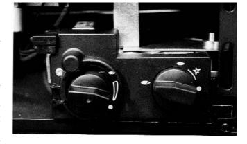
onds, release the knob and turn further to the left to the ON position. The main burner will light and be controlled in accordance with the main burner control knob setting. Adjust the main burner control knob to the desired setting.
