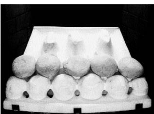
3. Take five more ceramic pebbles and position as shown to form the 'second row' of the fuel effect. The pebbles may be rotated as desired to fit into the gaps between the supports in order to create a random, realistic effect. Again, remember not to push the pebbles down too far into the valleys between the supports as this can have a detrimental effect to the flame picture.
