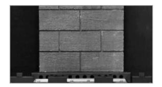
Place the ceramic combustion matrix onto the burner and the ceramic side cheeks onto the matrix.
