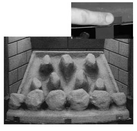
3. Open the bag of 16 moulded coals. All of the coals are the same. Take five coals and place them as shown. Care should be taken to ensure that the coals bridge the gap between the front coal and the four coal supports at the front of the matrix. Care should also be taken not to push the coals right down between the coal supports, as this can detract from the flame picture when the appliance is running.
