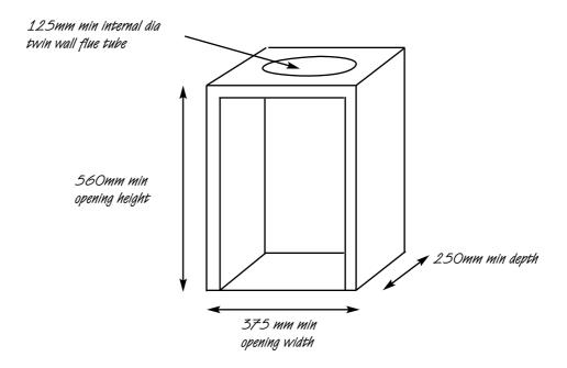
Some flue boxes may require minor adaptation when fitting the fire using the cable fixing kit. The firebox, base of the flue box, and the hearth may be drilled to allow plugs and screws to secure installation.
