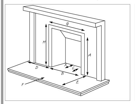
A. Opening height: 545mm min/575 mm max.B. Opening width: 390mm min/440mm max. C. Mounting depth: 250mm D. Hearth must extend minimum of 150mm either side of the opening. E. Hearth must extend minimum of 300mm in front of the opening. F. Non-combustible hearth must be a minimum of 50mm in height, or be surrounded by 50mm high fender. G. 470mm, this area must be flat and vertical to ensure a good seal. H. 585mm, this area must be flat and vertical to ensure a good seal.
