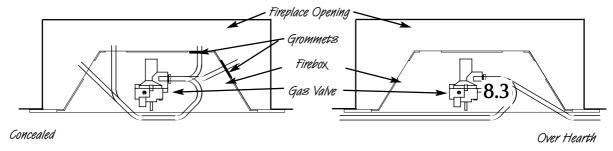
If using an across the hearth connection, then the firefront is notched and the supply pipe can be routed through this.
