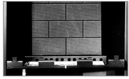
Place the ceramic combustion matrix onto the burner and the ceramic side cheeks onto the matrix.
