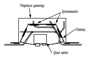
If using a concealed supply it should be laid in accordance with the diagram below. Select the supply route most relevant to the entry point of the gas supply into the fireplace opening. If using an across the hearth connection, then the firefront is notched and the supply pipe can be routed through this.
