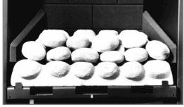
Place the middle row of four pebbles onto the supports in the matrix, over the top of the holes. Ensure the pebbles are not turned sideways, such that they actually enter the holes.
