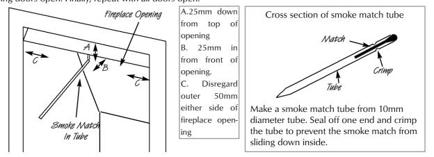
NOTE: If spillage is still indicated after undertaking all of the above, there may be a problem with the flue setup, or insufficient ventilation is present.
