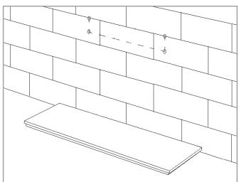
The lintel should be inserted and securely slate pinned, leaving the wall above safe and firm.
