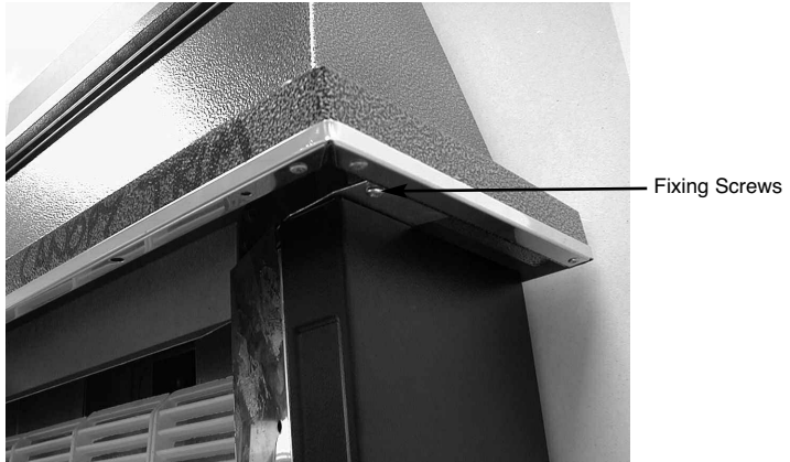
Fig. 6 Removing the Upper Outer Case Fixing Screws
