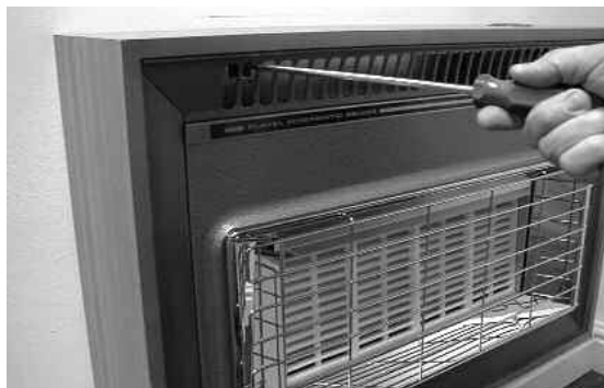
Fig. 10 Removing the Upper Outer Case Fixing Screws
