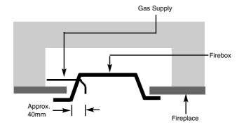
Note: Before breaking into the gas supply a pressure drop test should be carried out to establish that the existing pipework is sound.
