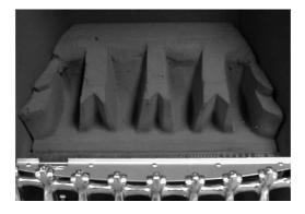
b) Position the two halves of the front ceramic (L/H & R/H) on the locating channel in the front ceramic, ensuring it is located onto the lip on the burner front ceramic support. (See fig. 11 below)
