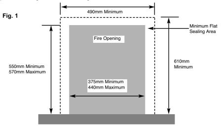
When installing into a brick built chimney, you must ensure that there is sufficient depth to accommodate any debris which may fall from the chimney. This depth must be sufficient to accommodate 12 litres of volumetric space.
