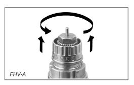
Danfoss pre-settable valve bodies incorporate easy setting adjustment rings with clearly engraved setting markers scaled from  $\bf 1$  -  $\bf 7$  and  $\bf N$ . Setting values can be set quickly and precisely, without the need for tools, as follows:
