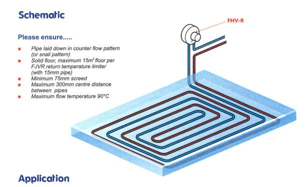
A self-acting return temperature limiter for controlling the floor temperature of individual rooms.
