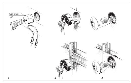
FHV valves are equally suitable for installation in solid or partition walls. To assist in the fitting of FHV control valves, we offer a compact customised valve enclosure wall box that can be fitted and fastened easily into a shallow recess in any type of wall.
