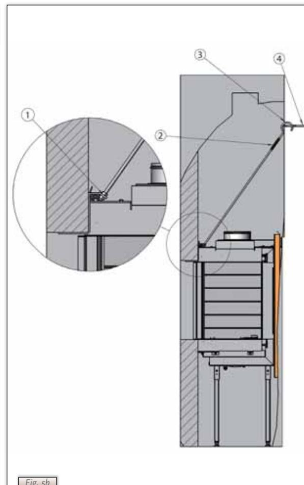
**!Caution** Do not allow the mantel iron to rest on the flanges of the build-in frame.
