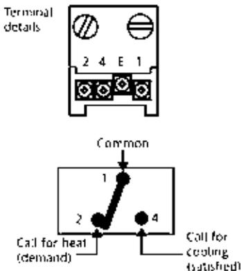
For boiler frost protection using PTS1 in conjunction with a standard frost thermostat:
