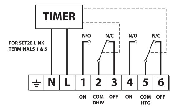
**NOTE**: For mains voltage applications links must be fitted between terminals L and 2 and between 1 and 5.
