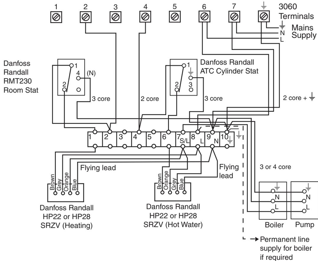
NOTE: This unit is NOT suitable for use with fully motorised zone valves requiring both ON and OFF electrical signals when used in the heating circuit
