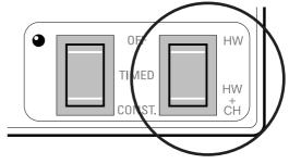
HW - heating is turned off and only the hot water is controlled according to the set programme.
