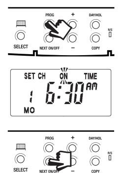
Continue programming the heating/hot water **ON** and **OFF** times by pressing:
