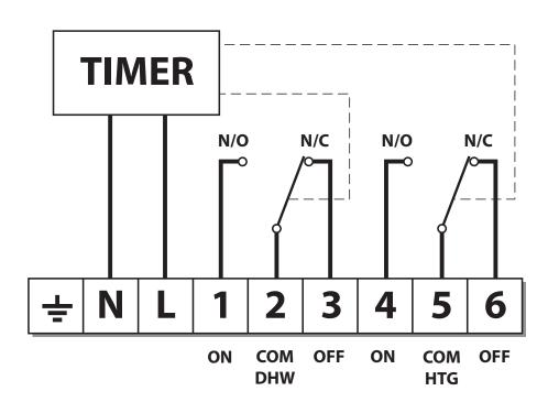
**NOTE**: For mains voltage applications links must be fitted between terminals L, 2 and 5.
