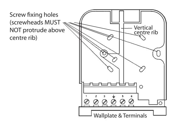
4. Surface cables can only enter from below the unit. Cut an appropriate cable aperture in the wiring cover. If the wallplate is mounted on a plaster box, cables can enter from the rear below the terminal block.
