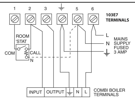
Note: Connection — — — — must only be made if input/output of boiler are 230V signals
