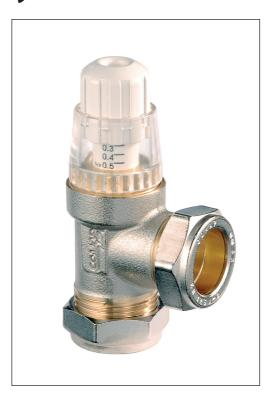
The ARV22 is an automatic by-pass control valve intended for use in domestic central heating systems. Its function is to allow a minimum flow to be maintained through the boiler as the water flow through the pump is reduced by, for example, radiator thermostats. The ARV22 automatically opens and closes depending on system load.
