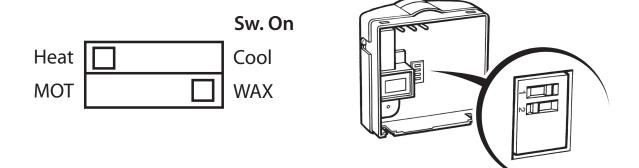
**HEAT** - proportional output will activate if temperature is below the setpoint. Frost protection mode is available (see page 10).
