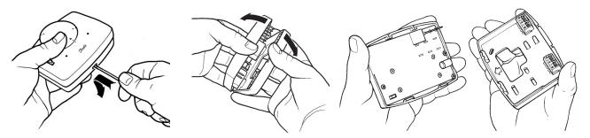
□ Fix at a height of approximately 1.5m from the floor, away from draughts or heat sources such as fan-coil outlets, sunlight or office equipment.
