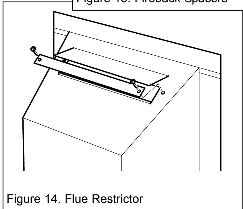
Figure 14. Flue Restrictor
