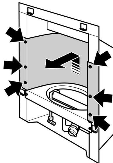
Figure 42. Removal of Inner reflector
