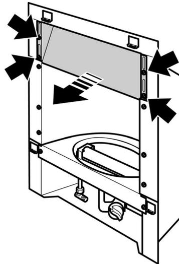
Figure 41. Spillage plate removal
