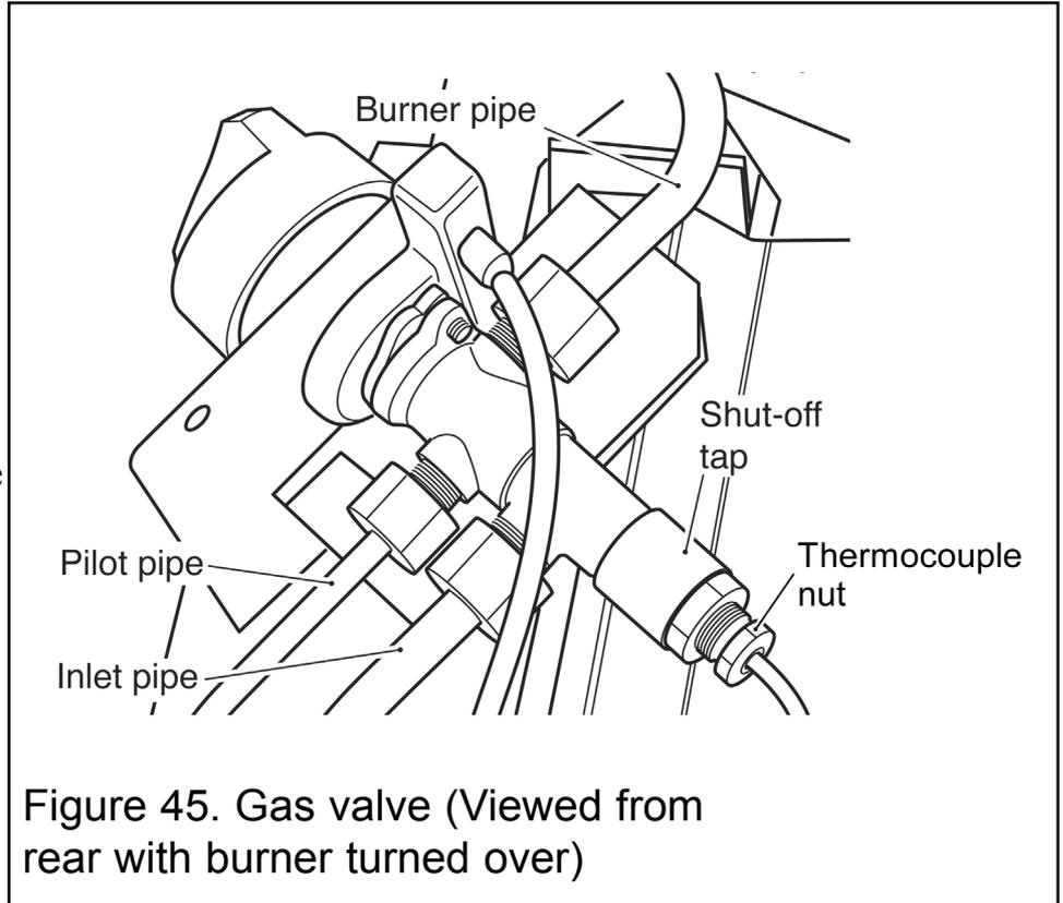
Figure 45. Gas valve (Viewed from rear with burner turned over)
