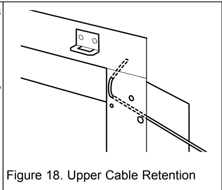
Figure 18. Upper Cable Retention
