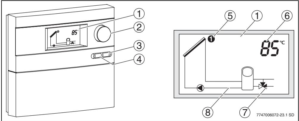
Fig. 37 Controller and display
