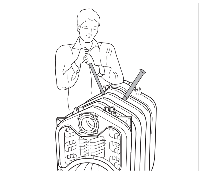
Fig. 26 Separate the boiler block
